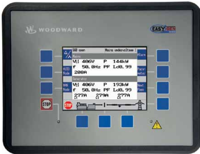
The easYgen-3400/3500 models expand the functionality of Woodward’s easYgen-3000 series by providing additional CAN communication capability to LS-5 series circuit breaker controls. The easYgen-3500 model shown here is panel door mounted and features a 14.5 cm diagonal, back-lit color LCD screen.
